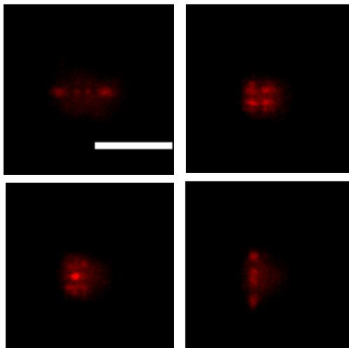
**Figure 10: Tetrapod PSF with the addition of dielectric phase mask to the optical path.** Yeast cells in a logarithmic phase in SC-LFM (2% glucose) growth medium were visualized under an inverted fluorescent microscope with a dielectric phase mask. Localized tetrapod PSF in different Z positions in YS0042 yeast strain bearing the LexA system with iRFP720 fluorescent protein at URA3 locus. Each PSF shape encodes the depth of the localized spot. Scale bar- 5 $\mu$ m.
