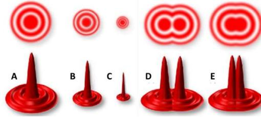
**Figure 3: Airy disk PSF illustration.** The Airy disk size depends on the objective numerical aperture (NA). (A) wide profile due to low NA; (B) moderately wide profile due to moderate NA; (C) narrow profile due to high NA; (D) Airy disk intensity profile for emitters in the limit of resolution; (E) PSF for emitters in very close proximity with overlapping center, obtains single unresolved localization
